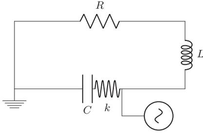
FIG. 1. The lumped-element representation of a  $RLC$  circuit where one of the capacitor plates is a vibrating drum. This plate is mechanically driven so that the effective distance  $d_0 + x$  between the plates of the capacitor is varied. A resistor was included to depict the unavoidable dissipation affecting the circuit.
