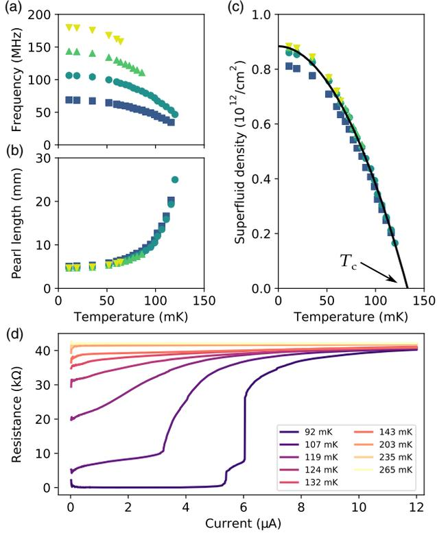
FIG. 2. Temperature dependence of the superfluid characteristics. (a) Frequencies of the cavity modes from  $m = 2$  (blue squares) to  $m = 5$  (yellow reversed triangles) at  $V_{BG} = 0$  V. (b) Pearl length and (c) superfluid density calculated from the data in (a) using Eqs. (1) and (2). The solid line in (c) is the best fit of Eq. (3) for  $m = 3$ , which gives  $T_c = 133 \pm 2$  mK. (d) Resistance-current characteristics measured on the ground plane.
