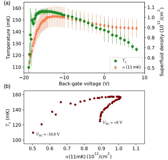
FIG. 4. Analysis of the superfluid gate dependence. (a)  $T_c$  and  $n(11 \text{ mK})$  as a function of  $V_{\text{BG}}$ .  $T_c$  is calculated by fitting the data from Fig. 3(c) with Eq. (3). (b) Critical temperature as a function of the superfluid density at 11 mK.
