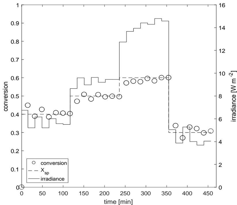
**Fig. 4 Dynamic development of the toluene conversion (controlled variable) and irradiance (manipulated variable) during a set-point tracking experiment in closed-loop mode with feedback control (Experiment#1).**
