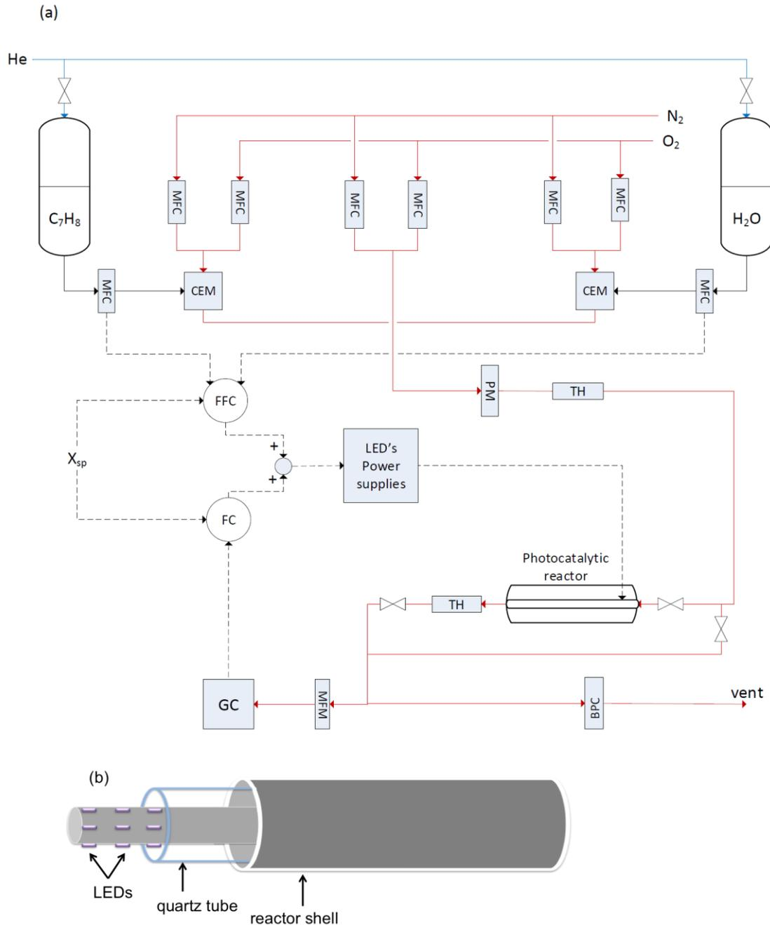
**Fig. 1 (a) Flow diagram of the experimental setup. MFC - Mass Flow Controller; BPC- Back Pressure Controller; CEM - Controlled Evaporator Mixer; TH- Thermo Hygrometer; PM- Pressure meter; FC- Feedback Controller; FFC-Feedforward Controller;(b) the structure of the photocatalytic reactor.**
