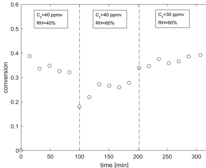
**Fig. 6 Toluene conversion during three different operating conditions at a constant irradiance of 6.5 [W m<sup>-2</sup>] and flow rate of 1020[ml min<sup>-1</sup>] in open-loop mode (Experiment #3).**
