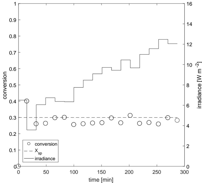
**Fig. 5 Dynamic development of the toluene conversion (controlled variable) and irradiance (manipulated variable) during a disturbance-rejection experiment in closed-loop mode with feedback control (Experiment#2).**
