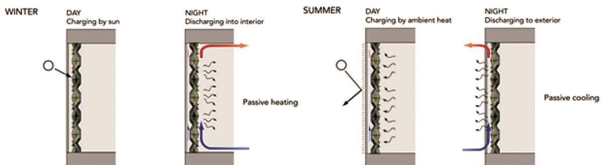
Figure 1: Winter (heating) and summer (cooling) mode of the Trombe wall.
