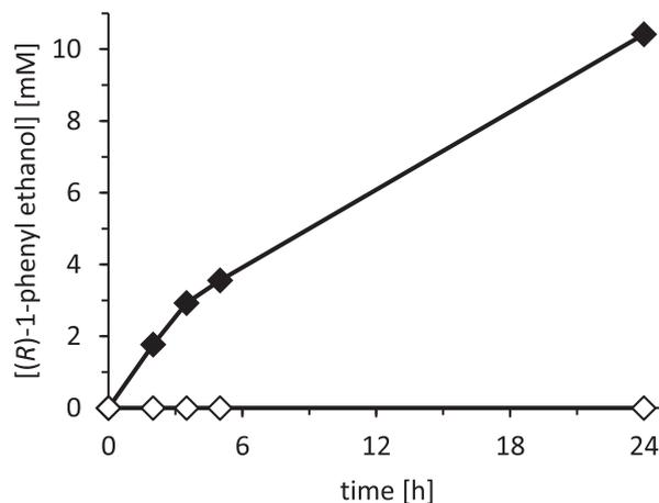
**Fig. 1.** Representative time course of the bienzymatic hydroxylation of ethyl benzene (Scheme 1) using purified (◆) or crude (◇) AoFOx preparations. Conditions: KPI buffer (100 mM, pH 6), [rAaeUPO] = 200 nM, [AoFOx] = 20 nM, [ethyl benzene] = 10 mM, [NaHCO<sub>2</sub>] = 100 mM, T = 30 °C.
