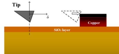
Fig. 5: Explanation of delamination test for Cu dot on SiO<sub>2</sub> substrate with lateral loading.
