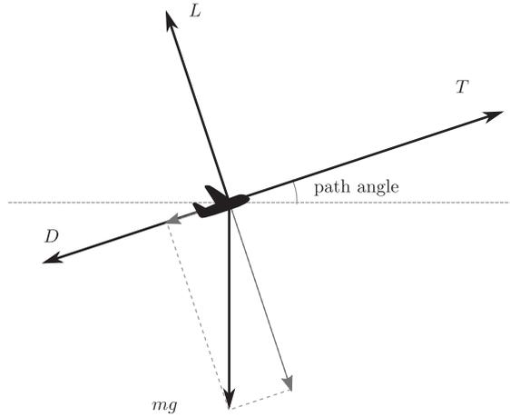
Fig. 2. Forces acting on an airborne aircraft (climb).
