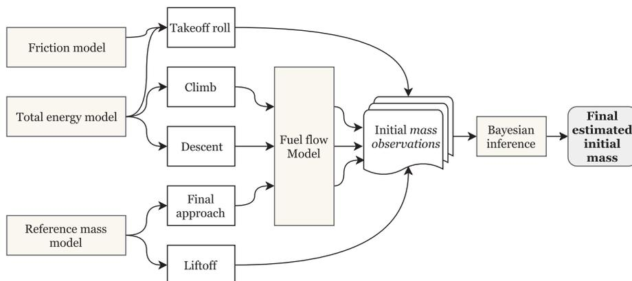
Fig. 1. Flow chart of the estimation structure.
