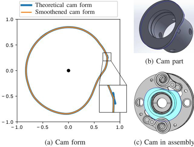
Fig. 5: Cam design for nonlinear spring transmission
