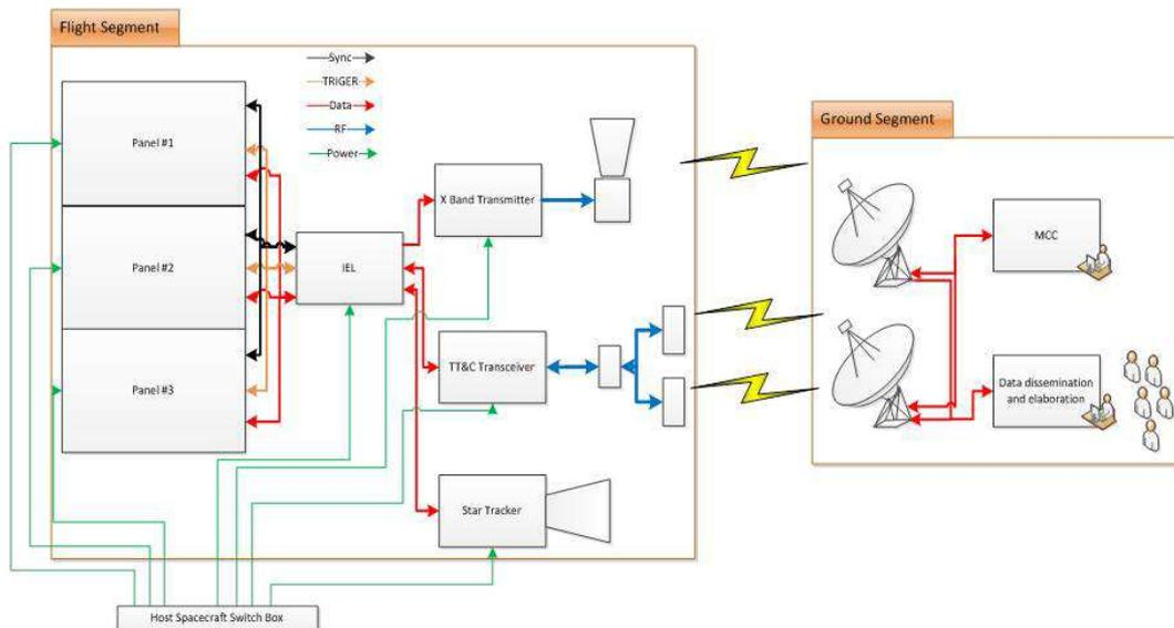
Figure 2. Overall System architecture.
