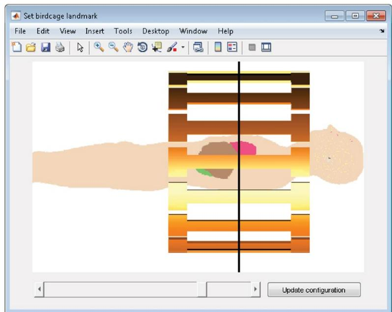
**FIGURE 3** The landmark of the birdcage can be selected, after which the corresponding electromagnetic fields are updated
