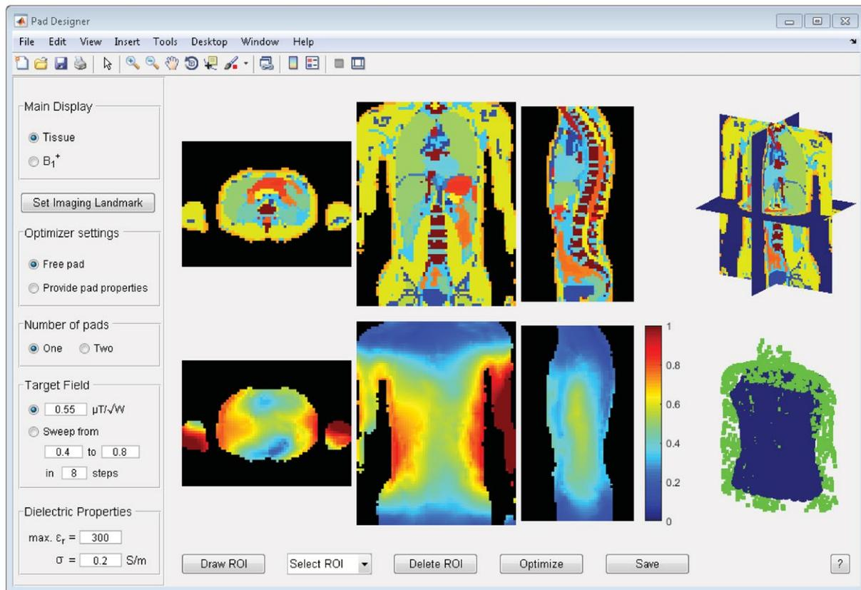
**FIGURE 2** Graphical user interface of the pad design tool. Tissue profiles are shown in the top row, whereas  $B_1^+$  fields are depicted in the bottom row. After a ROI is drawn, the user can start the optimization with the selected options
