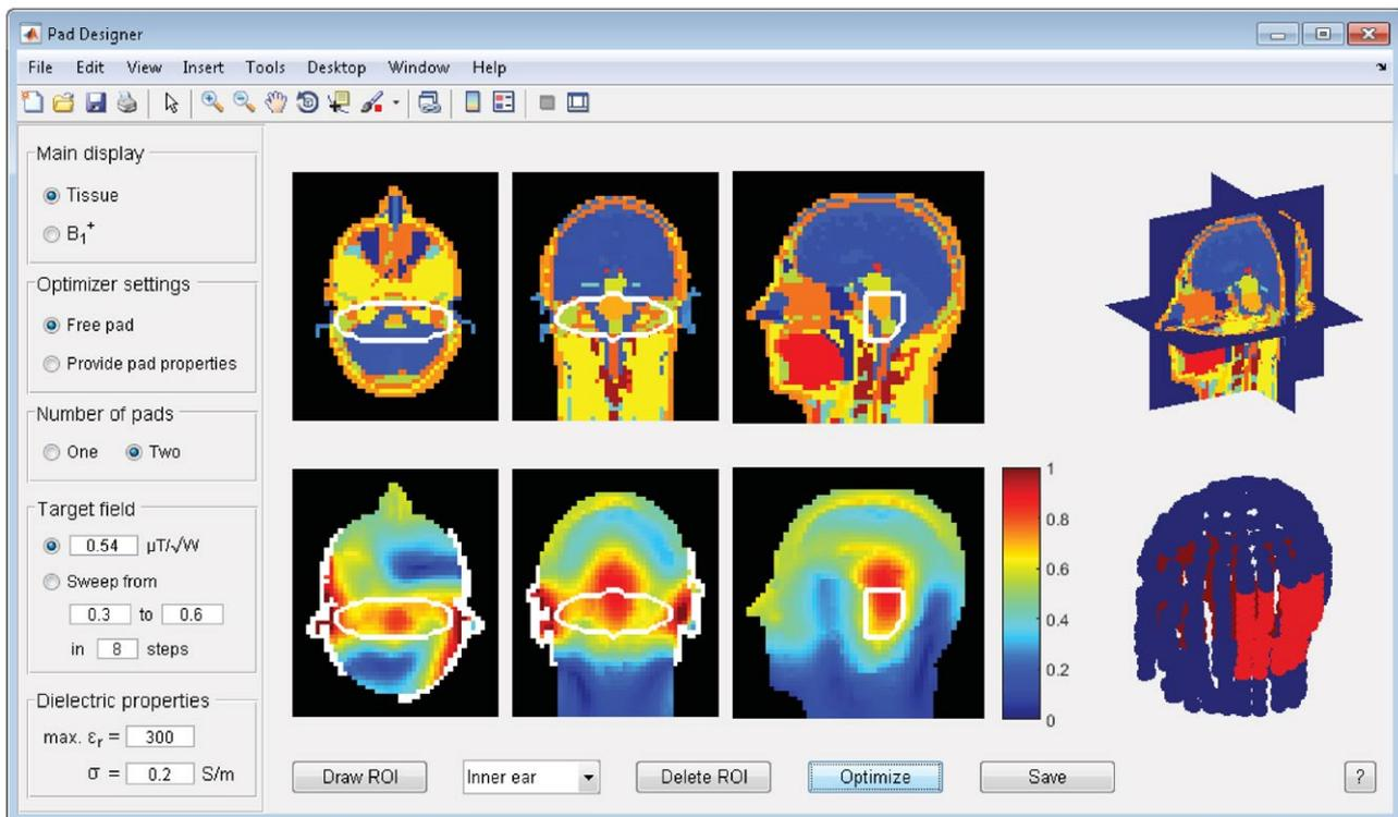
**FIGURE 5** Pad design results for the inner ear using 2 dielectric pads. The improved field and the location and dimension of the 2 dielectric pads are shown. The details on the improvement and the pad's parameters can be found in Supporting Information Figure S1
