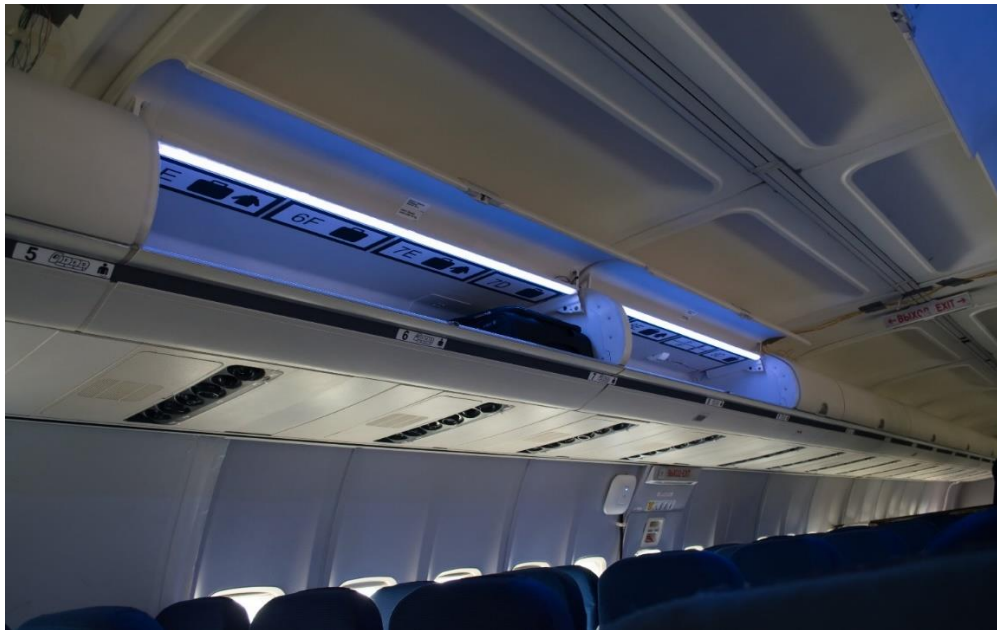
Figure 1. Screens and light strips in the overhead bins of the GHL system installed in B737 test fuselage.
