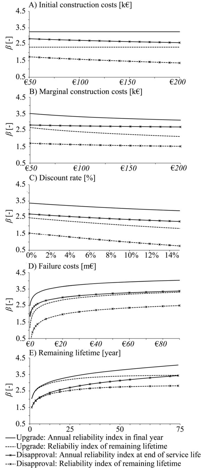
Figure 5: Sensitivity analysis 'repair' and 'upgrade' for  $Z_{\text{STR}}$  of scenario III. The reference calculation is based on:  $t_{\text{ref}}=25$ ;  $t_{\text{survive}}=50$ ;  $r=3\%$ ;  $L_{\text{eq}}=40\text{m}$ ;  $C_0=\text{€}100\text{k}$ ;  $C_m=\text{€}120\text{k}$ ;  $C_f=\text{€}5\text{m}$ .
