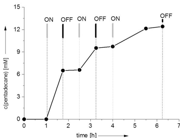
**Figure 1.** Photoenzymatic decarboxylation of palmitic acid into pentadecane. Conditions: [CvFAP] = 6.0  $\mu\text{M}$ , [palmitic acid] = 13 mM, Tris-HCl (pH 8.5, 100 mM), 30% DMSO, illumination with blue light.
