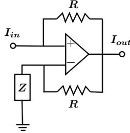
Figure 12: Negative-impedance converter
