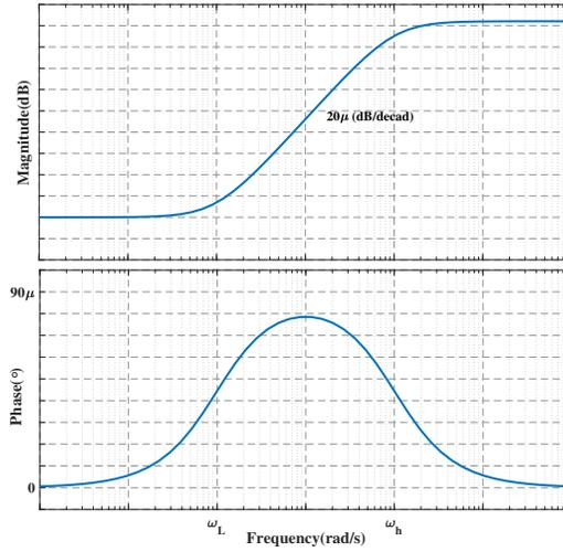
Figure 4: Bode diagram of FO-lead compensator
