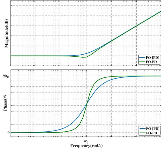
Figure 7: Bode plot of FO-PD and FO-[PD] controllers
