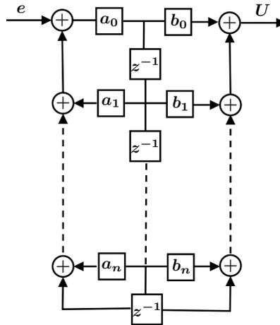
Figure 10: Block diagram of the canonical representation
