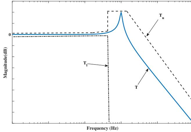
Figure 9: Frequency domain constraints on complementary sensitivity function
