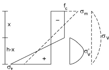
Stability design thus is a common second order strength calculation. The solutions of the second order equilibrium equations have to satisfy the failure criterion. This failure criterion is therefore essential and as shown in **A(2009)**, for statically indeterminate structures, and for combined loading, the idealized linear elastic calculation applied for failure, as given by the dashed lines in Fig.D-8, is not sufficient to describe and predict strength behavior and
