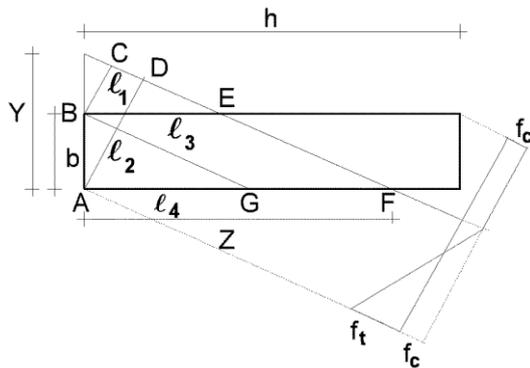
The assumption of all existing models for combined bending and compression loading, that a specific compression strain limit is determining for failure is shown to be incorrect. For instance, it predicts from the compression failure that there is no size effect of the strength. The measurements and theory show that there always is a size effect at any value of  $s$  and for any load combination because the bending tensile strength is always
