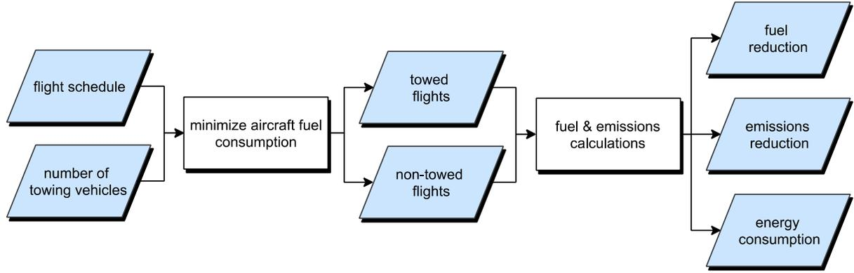
**Figure 2: Determining fuel, emissions and energy savings**
