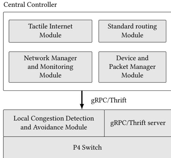
Figure 1: Hierarchical design of the control plane.
