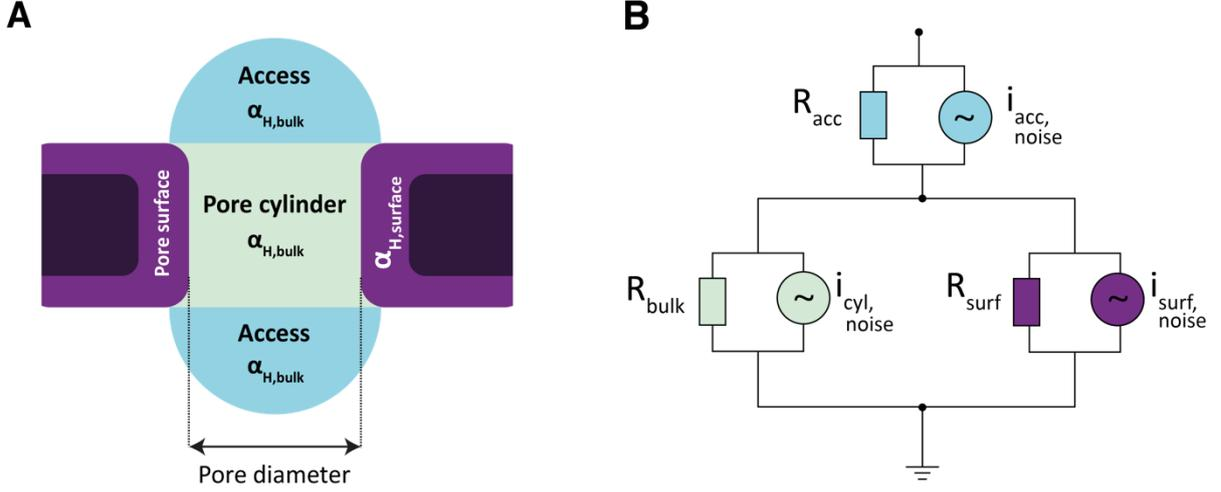
**Figure 1.** (A) Schematic representation of the relevant nanopore regions: access region (blue), pore-cylinder region (green), pore-surface (purple). (B) Equivalent circuit of the nanopore sensor. Nanopore regions are modelled as resistive elements connected in parallel to noise current generators.
