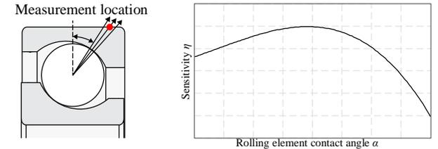
Fig. 2. Schematic representation of relationship between contact angle and measurement sensitivity  $\eta$
