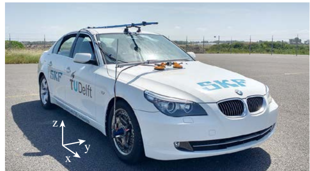
Fig. 9. The instrumented test vehicle including load sign convention
