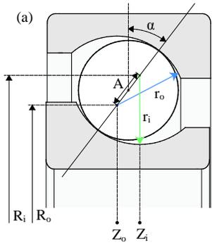
Fig. 4. Bearing section view showing bearing parameters
