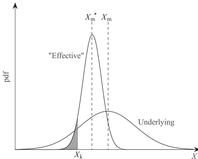
**Figure 1.** Derivation of characteristic property value satisfying EC7: underlying distribution of  $X$ , and “effective” distribution accounting for influence of spatial correlation and problem being analysed.
