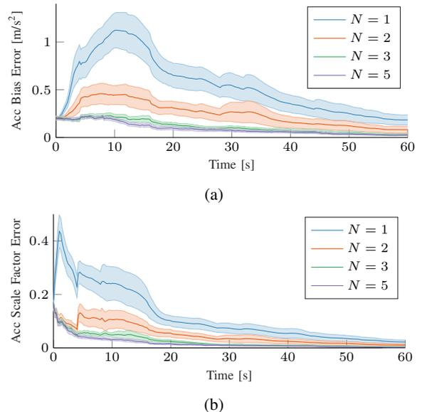
Fig. 4: Evolution of error for estimating accelerometer biases (a) and scale factors (b) over time using an uncertain initial orientation for different horizons lengths  $N$ . The mean error over all datasets is visualized using the solid line and the corresponding standard error using the colored patch.
