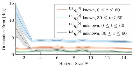
Fig. 3: Comparison of the orientation error for different horizon lengths  $N$  using a perfect and an uncertain initial guess. The mean RMSE over all datasets is visualized using the solid line and its standard error using the colored patch.
