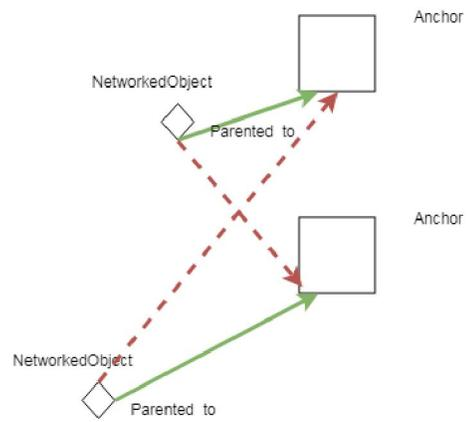
Figure 7: Spatial functioning of the anchor parenting system: *green arrows* mean that the game object is parented to that anchor, *red lines* mean that the distance is too large and the object is not parented to that anchor
