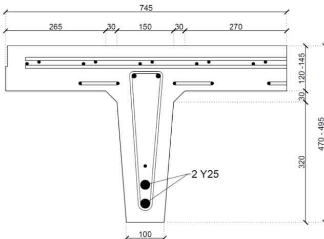
Figure 1. T-beam cross section. Units: mm.
