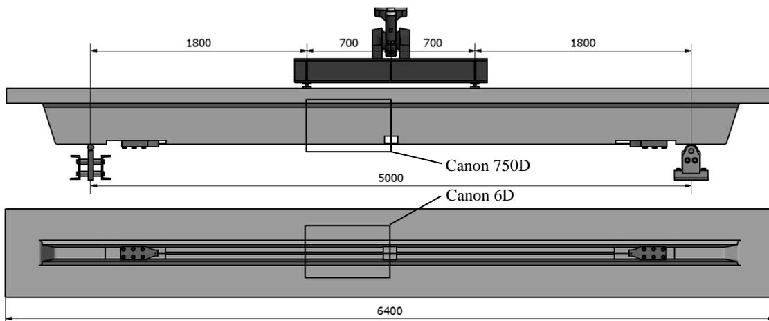
Figure 2. Test beam and DIC setup. Units: mm.
