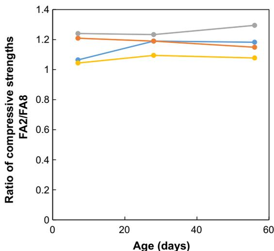
**Fig. 5** Ratio of mean compressive strengths within each laboratory between FA2 and FA8 at each age, for laboratories that returned valid results for both concretes. Each line represents one laboratory
