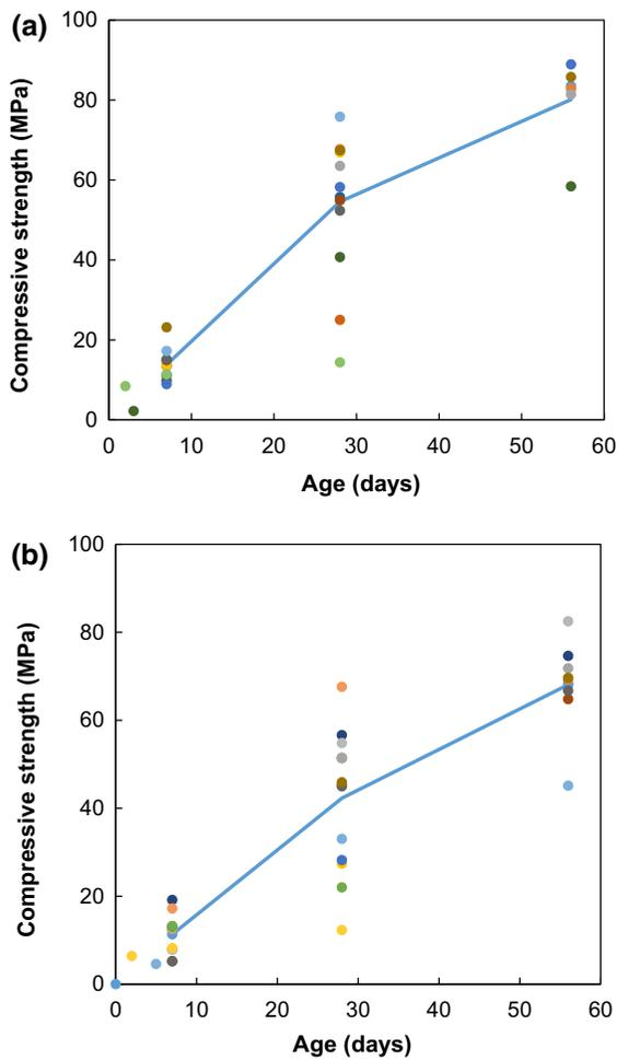
**Fig. 4** Compressive strengths determined for fly ash-based AAM concretes cured under sealed conditions at 20–25 °C: **a** FA2, and **b** FA8. Each point represents a single reported result; each laboratory returned between 1 and 6 strength result(s) per age; not all laboratories returned results for each mix at every age. The solid line represents the mean of all reported data
