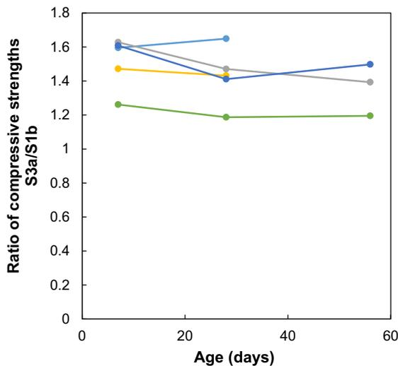
**Fig. 3** Ratio of mean compressive strengths within each laboratory between S3a and S1b at each age, for laboratories that returned valid results for both concretes. Each line represents one laboratory
