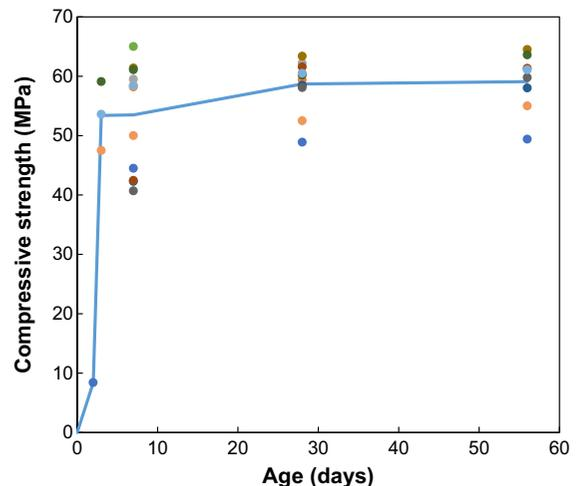
**Fig. 6** Compressive strengths determined for metakaolin-based AAM concretes cured under sealed conditions at 20–25 °C. Each point represents a single reported result; each laboratory returned between 1 and 6 strength result(s) per age; not all laboratories returned results at every age. The solid line represents the mean of all reported data
