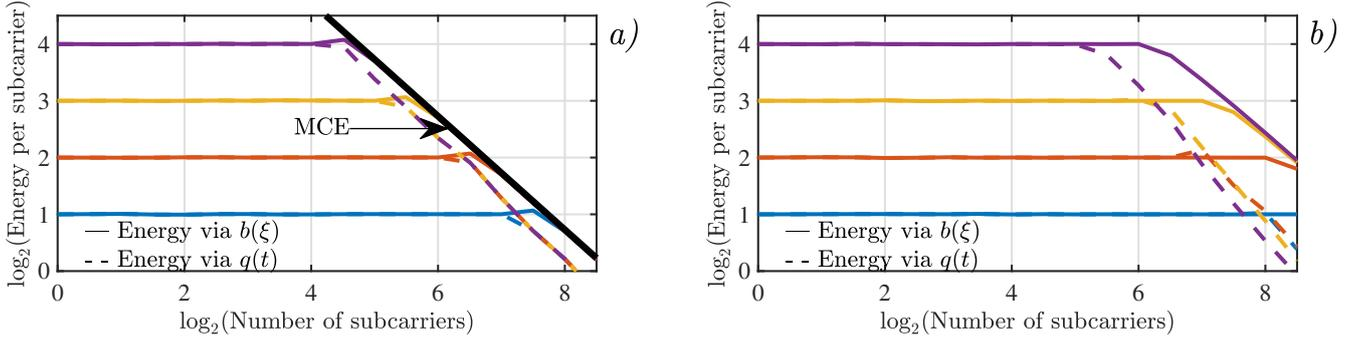
Fig. 1 *a)* PCCR: The two energy estimates agree almost upto the theoretical maximum. *b)* PCRb: The two estimates also start to decrease with number of subcarriers (signal duration) due to signal truncation and finite precision (similar to [12, Fig. 6a]).
