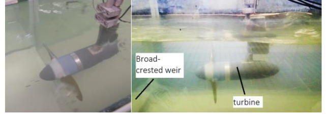
Fig. 3. The experimental set-up, consisting of a barrier weir with a two-bladed Tocardo Power Turbine (scale 1:9, rotor diameter = 0.4 m) in a flume of the Environmental Fluid Mechanics Laboratory of Delft University of Technology.
