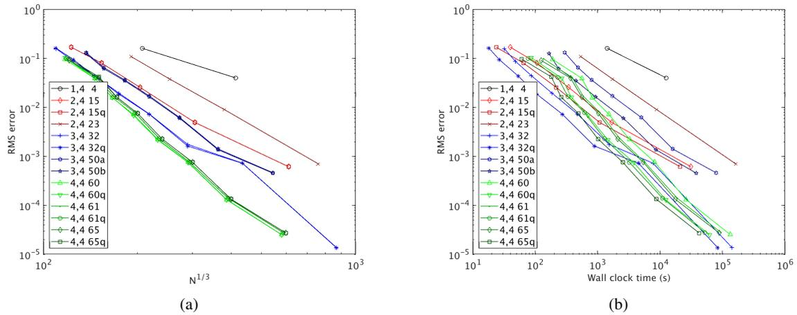
**Figure 1** RMS errors for a homogeneous elastic problem as a function of (a) the cube root of the number of scalar degrees of freedom  $N$  and (b) the elapsed wall clock time.
