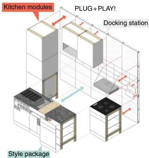
Figure 7. Concept design for the circular kitchen
