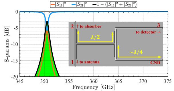
**Fig. 1.** Performance of an isolated filter designed to resonate at ~350 GHz with  $Q_f \sim 500$  simulated with Sonnet. In the inset the actual shape of the resonator.
