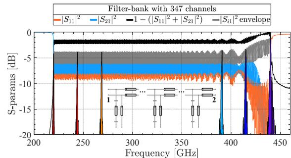
**Fig. 2.** Expected performance from the circuit model (see inset) of the filter-bank with 347 channels in terms of: reflections back to the antenna ( $|S_{11}|^2$ ), power dissipated in the termination ( $|S_{21}|^2$ ), and total power absorbed (no losses) by the detectors in the filter-bank ( $1 - |S_{11}|^2 - |S_{21}|^2$ ). The response of a few channels is displayed (colored peaks) for illustration. The gray line is the envelope of the most responding channel per frequency.
