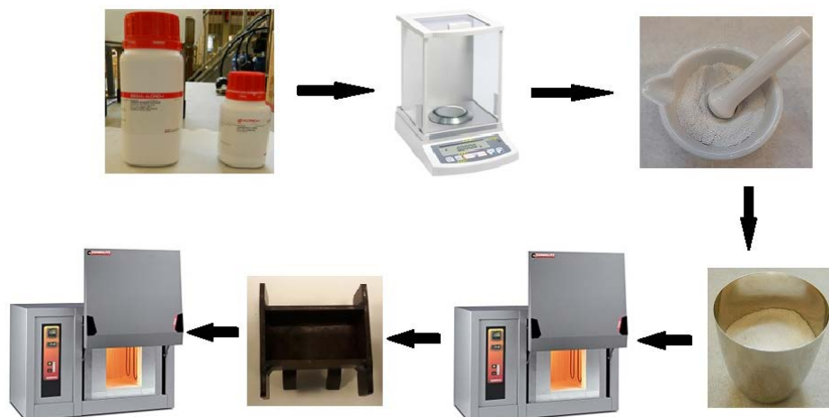
Fig. 1 Scheme of the glass samples production.
