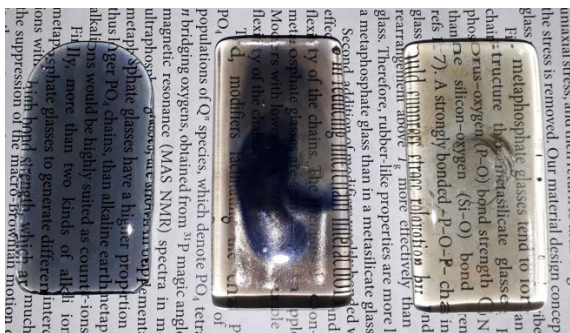
Fig. 5 Samples consisting of 12.5% slag melted at different temperatures: 1150°C, 1250°C, and 1350°C, respectively.
