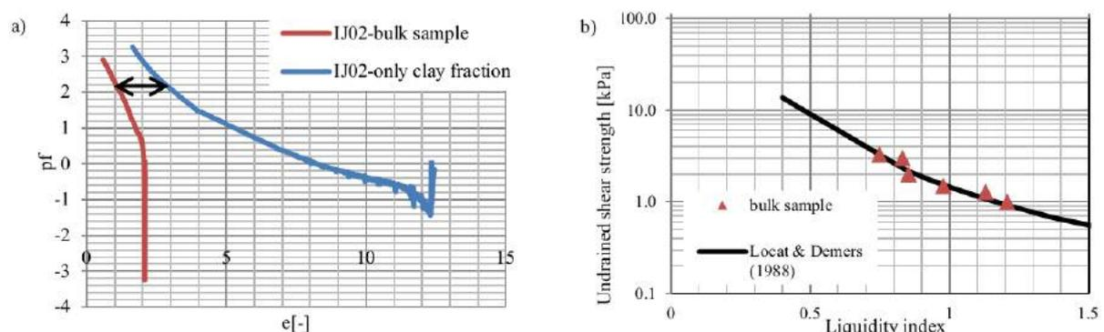
Figure 2. a) Water retention curve of a sieved and a natural sample of *Markermeer* Holocene clay. b) Correlation between the liquidity index and the undrained remoulded shear strength for a natural sample
