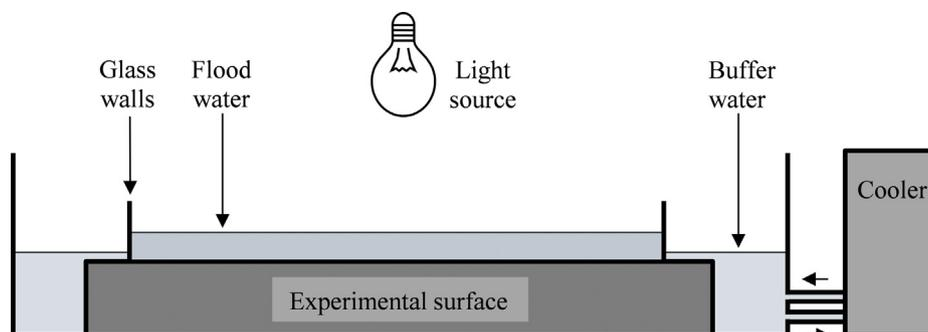
**Fig. 1.** Schematic representation of a reactor exposed to artificial light. Two such reactors were used in parallel. In the experiments under real sunlight the cooler was not used.
