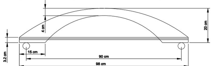
Figure 4: Test setup for reinforced concrete specimens 2
