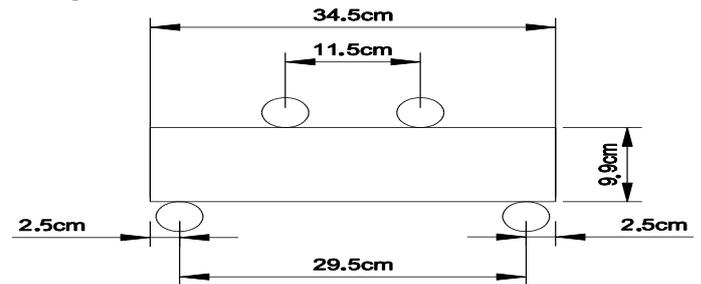
Figure 2: Test setup for beams 1-8
