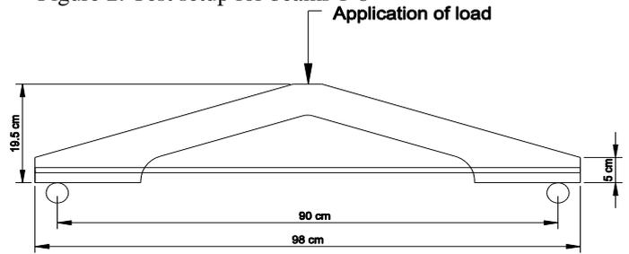
Figure 3: Test setup for reinforced concrete specimen 1
