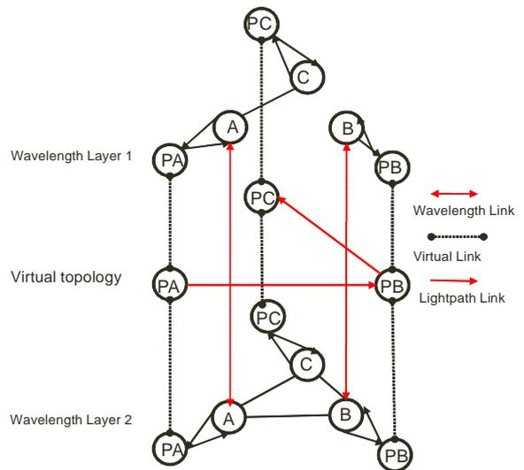
Fig. 5. Auxiliary graph for wavelength conversion
