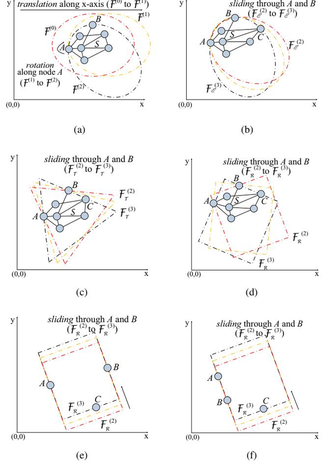
Fig. 2: (a) *Translation* and *Rotation*, illustrated for the ellipse; *Sliding* through  $A$  and  $B$  for: (b) an ellipse; (c) an equilateral triangle; (d) a rectangle if  $A$  and  $B$  lie on perpendicular sides; (e) a rectangle if  $A$  and  $B$  lie on parallel sides; and (f) a rectangle if  $A$  and  $B$  lie on a same side.
