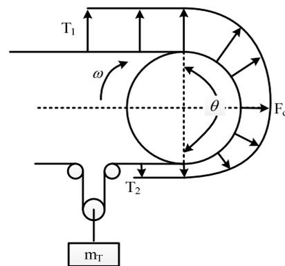
Fig. 1 Belt tension distribution in transient operation
