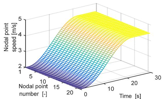
Fig. 8 Belt speed at each nodal point
