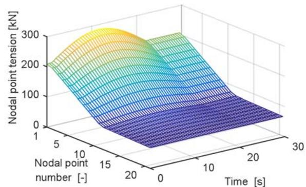
Fig. 7 Belt tension at each nodal point
