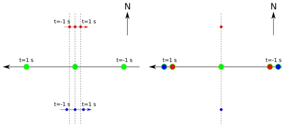
**Fig. 2** Illustration of the conceptual model. In the Earth-centered non-fixed reference system (left), the first burst (green) is received east of the last burst as Cryosat-2 is in a retrograde orbit. Due to Earth rotation, scatterers on the northside (red) and southside (blue) move at different
