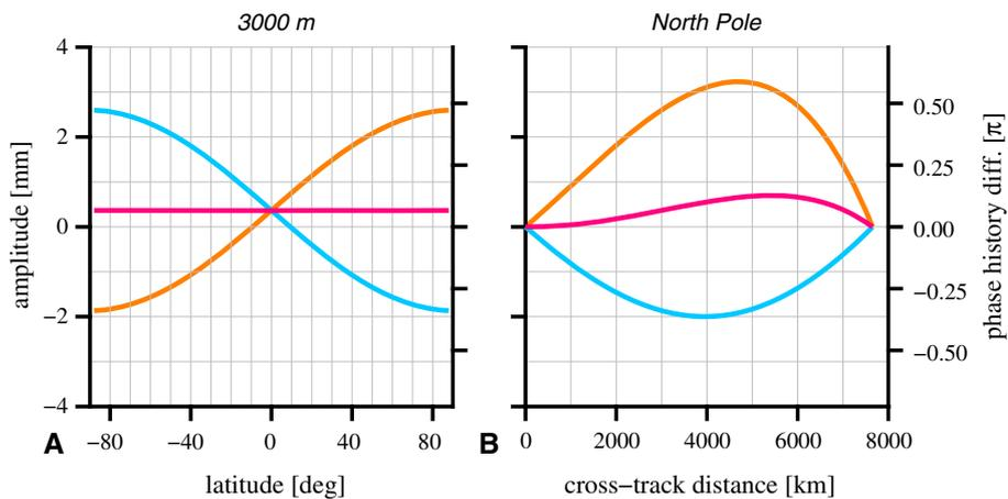
**Fig. 4** Modeled amplitudes of the range difference. In orange, the amplitude for a scatterer at the right side of the ground track and in blue on the left side. Positive values indicate a positive parabola, and negative values indicate a negative parabola. The pink line shows the geometrical effect on the range without Earth rotation for which is
