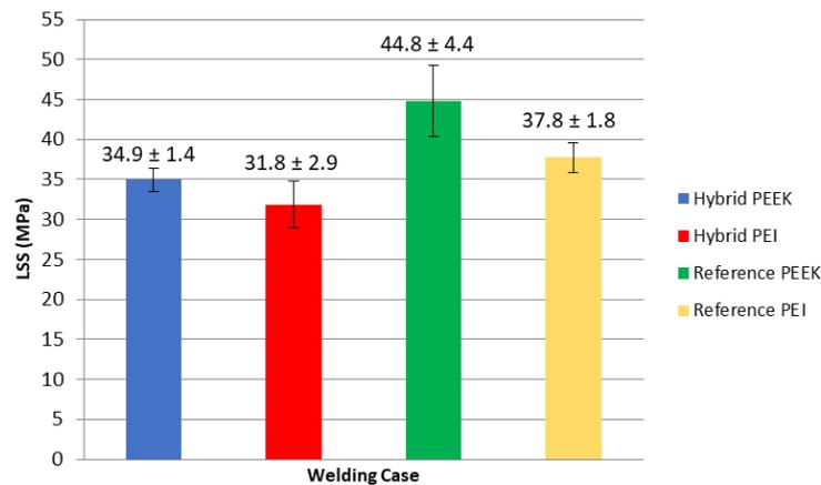
**Figure 2.** LSS values for the different welding configurations
