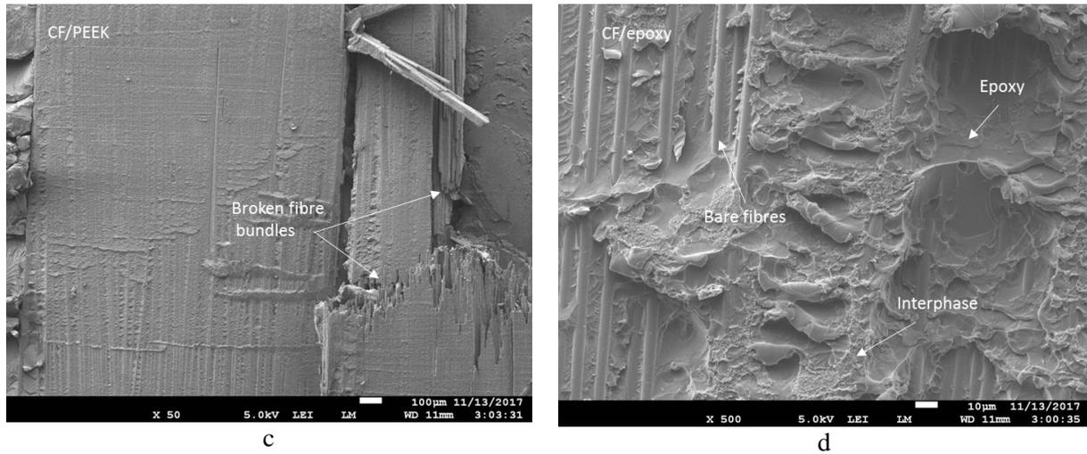
**Figure 3.** Representative fracture surfaces of a hybrid PEEK sample (a) and a hybrid PEI sample (b), showing unwelded areas and failure in CF/PEEK and CF/epoxy adherends, c) and d) are SEM images of the circled areas in a) showing failure in the CF/PEEK and failure in the CF/epoxy respectively.
