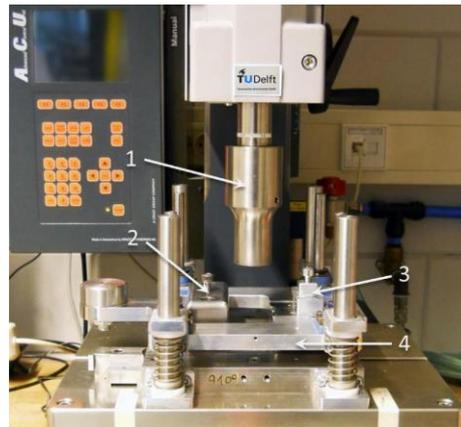
**Figure 1.** Custom made welding setup. 1: sonotrode, 2: clamp for the lower sample, 3: clamp for the upper sample and 4: sliding platform [9].
