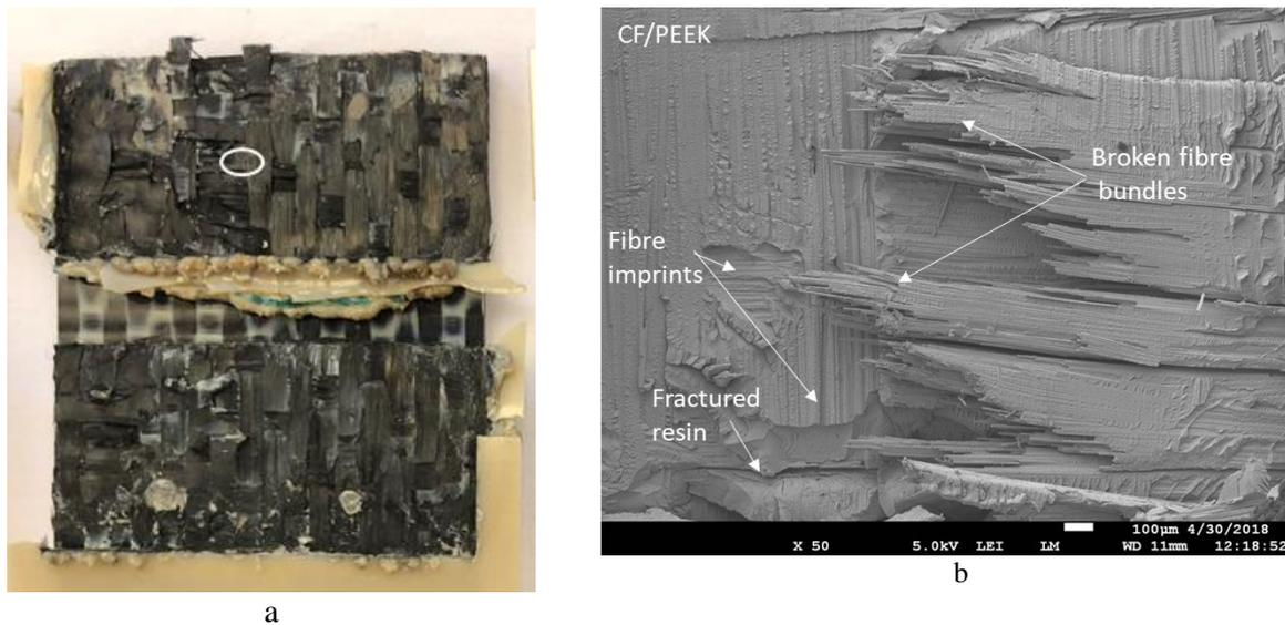
**Figure 4.** a) Representative fracture surfaces of a Reference PEEK sample showing failure deep into the composite and b) is a detailed SEM image of the circled area in a) showing broken fibres, fibre imprints and broken resin.
