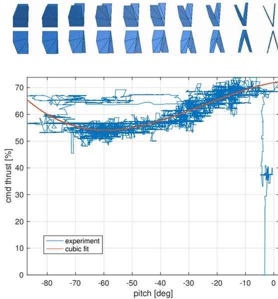
Figure 3: Throttle level against body pitch when flying in the wind tunnel with increasing wind speed and maintaining approximately levelled flight; experiment (blue) and cubic fit (red); the robot’s body posture is shown from top view.
