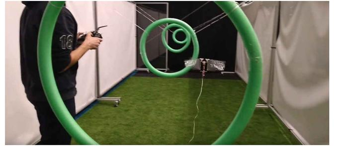
Figure 9: Flight through hoops - test setup.
