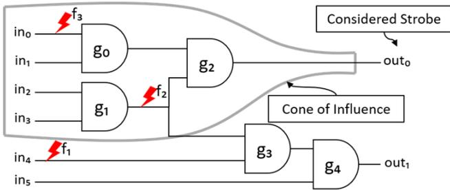
FIG. 1. STANDARD ANALYSIS EXAMPLE (CONE OF INFLUENCE ANALYSIS)
