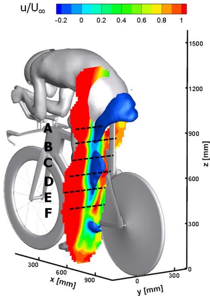
Figure 2: Cross-section of mean non-dimensional streamwise velocity in the near-wake of the stretched leg obtained at  $U_\infty = 5$  m/s. The dark blue iso-surface depicts a zero level of streamwise velocity.
