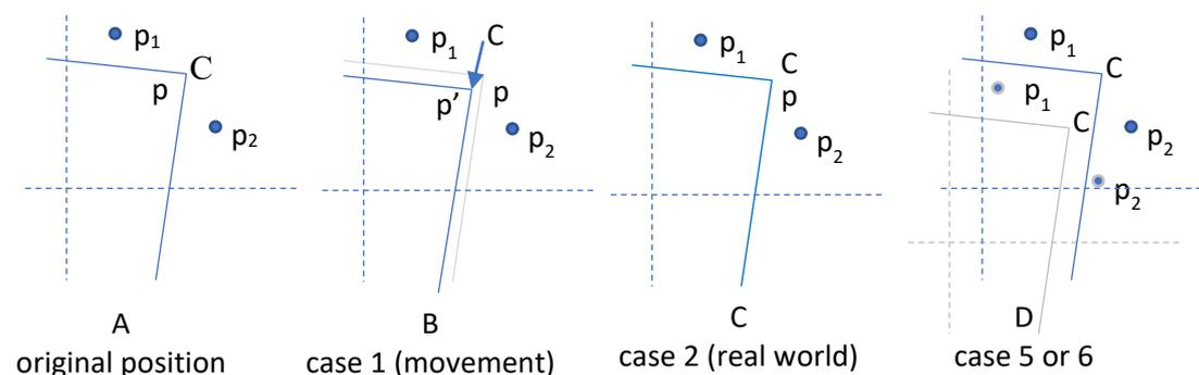
**Figure 2 Movements of a cadastral corner under various changes. Points p1 and p2 are assumed to be physical markers near the corner C. The location of C is marked as p. The two dashed lines indicate a local reference frame coordinate values.**
