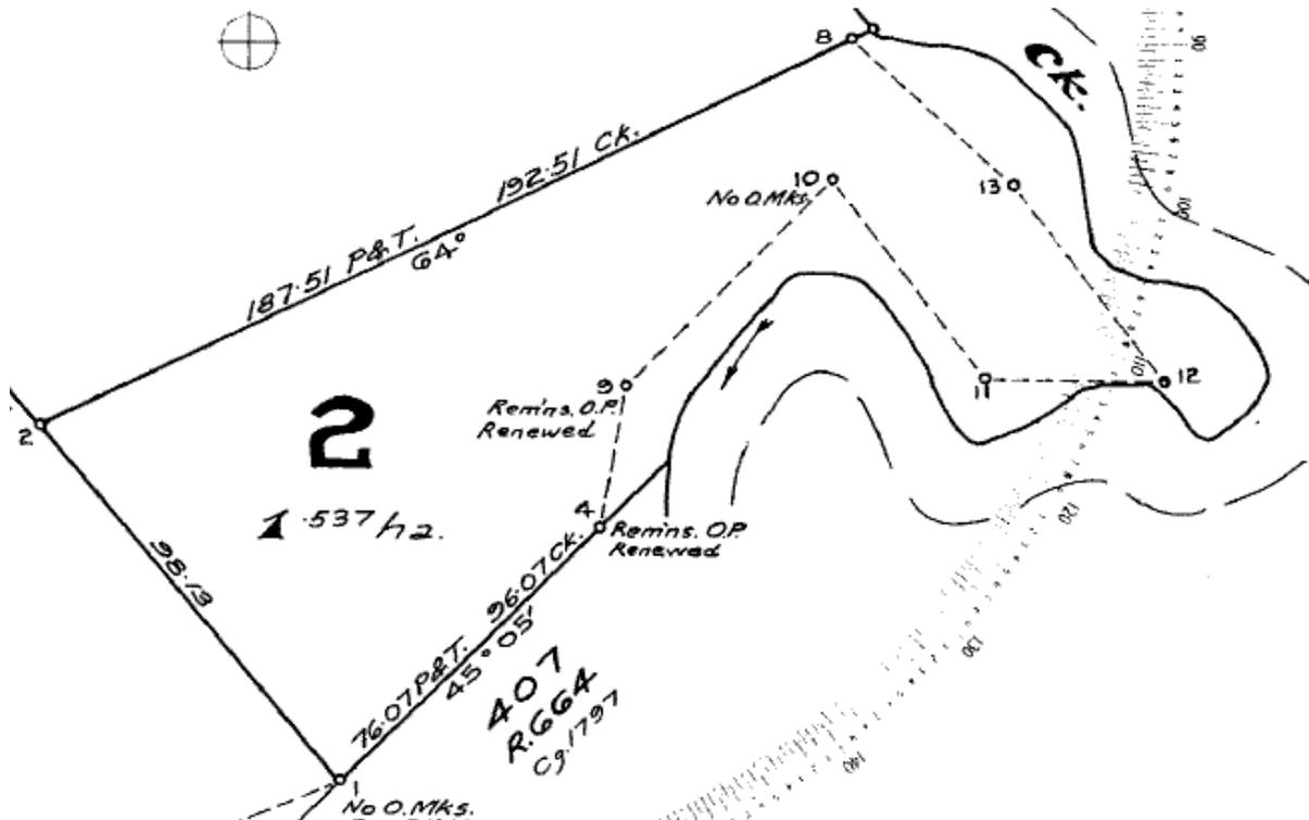
**Figure 8** Various point-like entities. Point 2 is a Node2D. Point 8 is a Vertex2D, but not a node in the cadastral fabric. Point 13 is a TraversePoint2D. The curved line is composed of a large number of Vertex2D objects which are on a natural boundary at an instant of time (in this case the plan date 9th Feb 1981).
