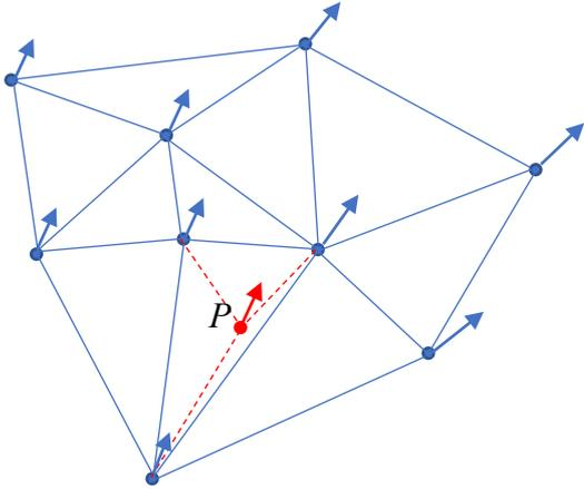
**Figure 3 A Vector TIN in 2D. The blue nodes are points at which the velocity (represented by the vector arrows) is known. The velocity at point P is interpolated from the vertices of the enclosing triangle.**
