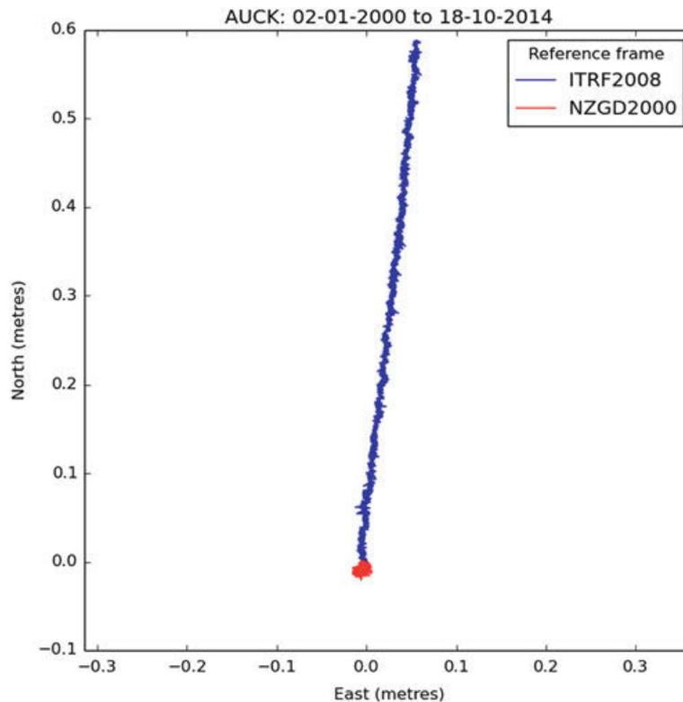
**Figure 1** Example of the trajectory of a PlateFixedLocation (a reference point in Auckland New Zealand) over a 15 year period. The position in relation to an ITRF is blue and red in relation to an LRF (NZGD2000). Note that “The trajectory in terms of the local frame is almost static”.
