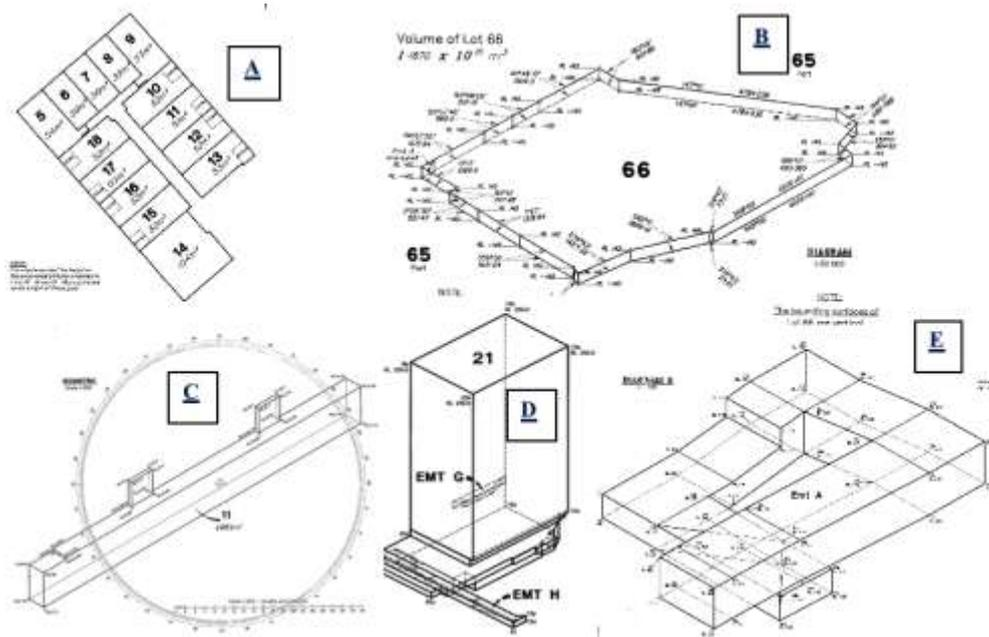
**Figure 7 — Subcategories of spatial unit geometries: A. Building Format spatial units; B. Simple Slice; C. Single-valued stepped spatial unit; D. Multi-valued stepped slice (“EMT G” forms a “cave”); E. General 3D spatial unit (Kalogianni et al., 2018)**
