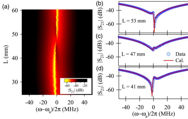
FIG. 2. (a) Transmission of the system ( $|S_{21}|$ ) as a function of  $\Delta_a$  and the separation between the two modes  $L$ . (b)–(d) Three typical spectra measured at  $L = 53$  mm,  $L = 47$  mm, and  $L = 41$  mm. Blue dots are experimental data and red solid lines are calculation results by using Eq. (11).
