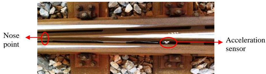
Figure 4: setup of measurement for acceleration of crossing nose
