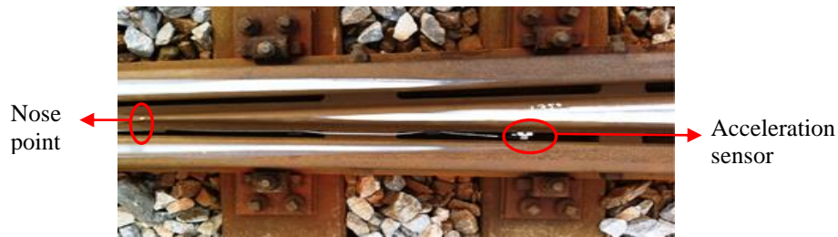
Figure 4: setup of measurement for acceleration of crossing nose
