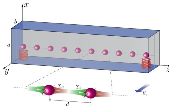
FIG. 1. Chain of magnetic spheres with period  $d$  in a microwave waveguide. The chain and waveguide are parallel to the  $\hat{z}$  axis and magnetizations are oriented along  $\hat{y}$  by a magnetic field  $H_y$ . Every magnet interacts with all other magnets to the right ( $\Sigma_R$ ) and left ( $\Sigma_L$ ). Small coils attached to each magnet can excite and detect the local magnon accumulation.
