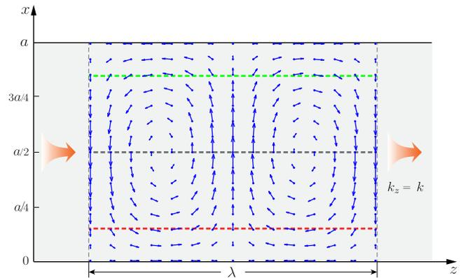
FIG. 2. Snapshot of magnetic-field vector distribution of the TE<sub>10</sub> waveguide mode over one wavelength  $\lambda$ . The green and red dashed lines indicate the chiral lines with (opposite) circular polarization.
