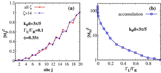
FIG. 4. Magnon accumulation excited by a phased antenna array with  $N = 20$  magnets. (a) The accumulation (squared magnetization amplitude) distribution over the magnets (red curve) is normalized by the largest value at the edge. The blue curve excludes the contribution of subradiant states. (b) Magnon accumulation as a function of chirality, normalized by its value for  $\Gamma_L/\Gamma_R = 1$ .
