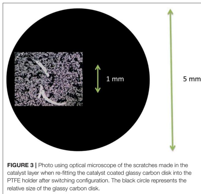
**FIGURE 3** | Photo using optical microscope of the scratches made in the catalyst layer when re-fitting the catalyst coated glassy carbon disk into the PTFE holder after switching configuration. The black circle represents the relative size of the glassy carbon disk.
