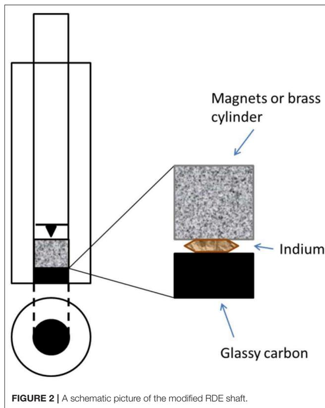
from 5 mm to 2 mm by ultra-fine polishing, thanks to *Surface Preparation Laboratory*, Zaandam, NL. A new, shorter shaft was made, keeping the spring-loaded tip to ensure good electrical contact with the magnets. The “cavity” inside of the modified RDE electrode was made such that it could accommodate either only magnets, only a non-magnetic brass cylinder or half-half magnets/brass as a crude way of varying the magnetic field strength. See **Figure 2** for a schematic illustration.
