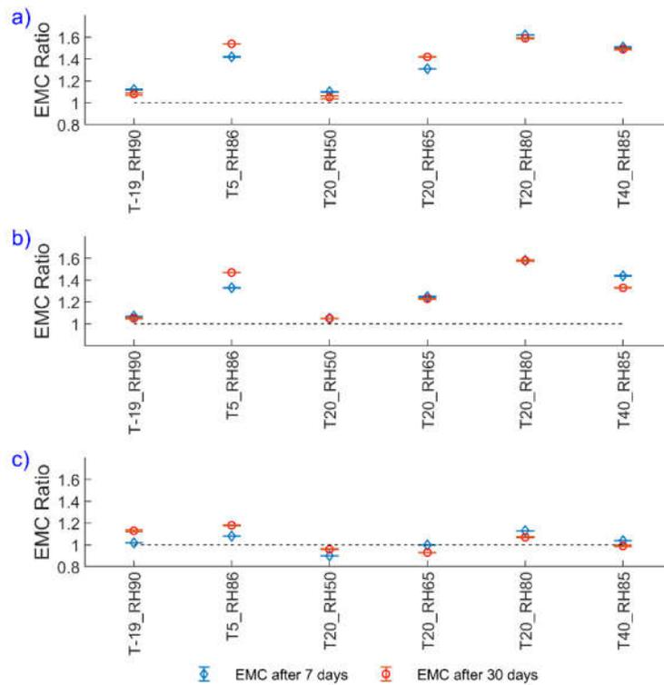
**Figure 2.** Equilibrium moisture content (EMC) ratio of pellets after 7 and 30 days of storage for (a) brown, (b) white, and (c) torrefied pellets. The error bars show the standard deviation and the dashed lines show the EMC for as-received pellets.
