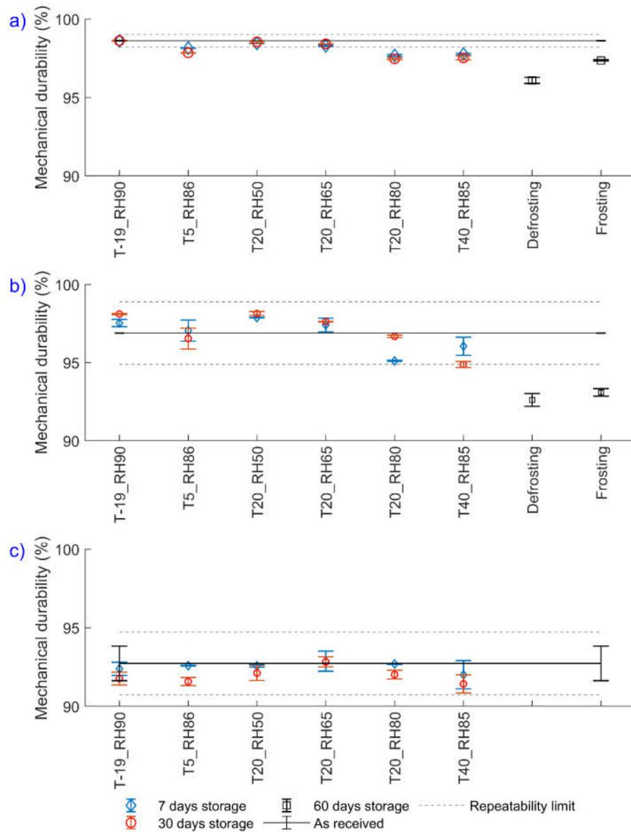
**Figure 5.** Mechanical durability values of different pellets after storage for (a) brown, (b) white, and (c) torrefied pellets. The error bars show the standard deviations and the solid lines show the as-received mechanical durability.
