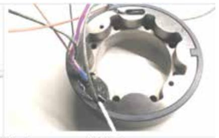
The iBearing sleeve with the sensors embedded.
