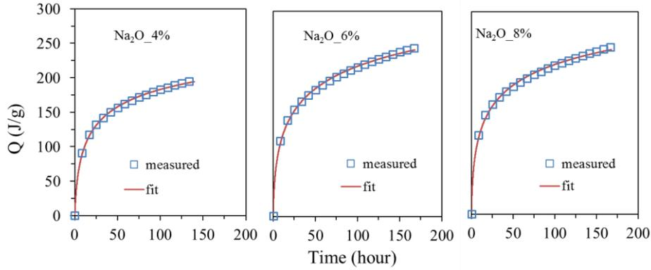
Figure 2: Exponential fits applied to the cumulative heat release for SHAS pastes. Symbols represent the experimental data points (1 out of 1000 shown) and the solid lines show the fit of Eq. (2) to the experimental data.
