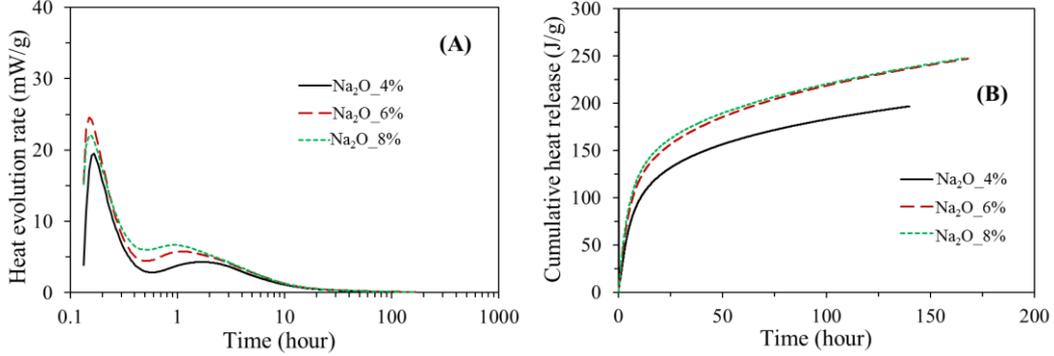
Figure 1: Heat evolution rate (A) and cumulative heat release (B) for SHAS pastes
